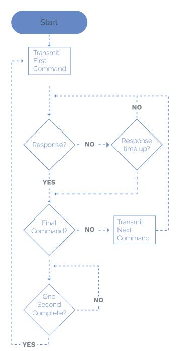
The intention of this protocol is to be low impact on the slave. If the slave fails to respond to requests, the Relay will try again in one second.
